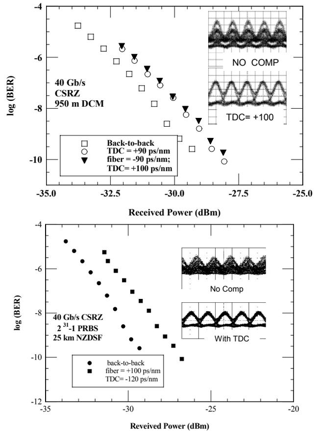
**Figure 3.** Measured bit-error-rates for 1549.32 nm: top (950m DCF) and bottom (25 km SMF) while the insets display the eye diagrams with and without the TDC. The left curve is the baseline.
