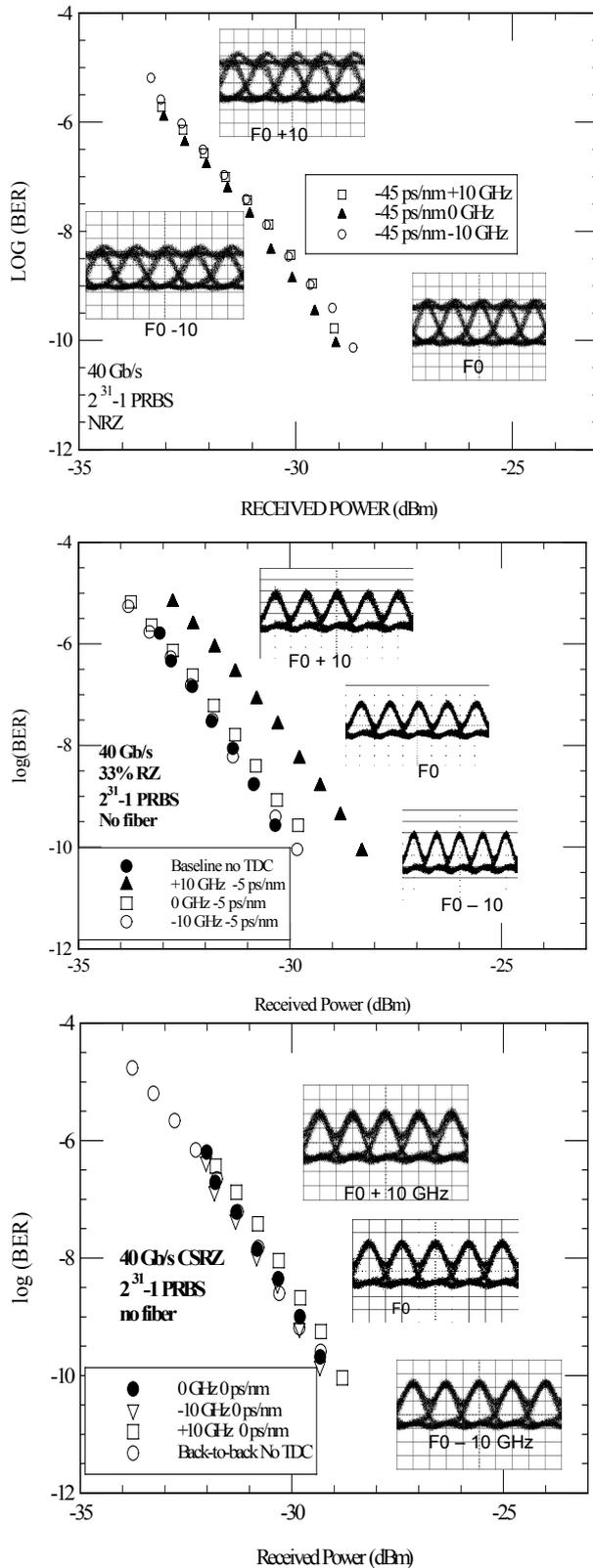
**Figure 2.** Measured bit-error-rate with center wavelength (193.5 THz or 1549.32 nm) detuning with the TDC set to (a) (top) -45 ps/nm (NRZ), (b) (center) -5 ps/nm (RZ) and (c) (bottom) 0 ps/nm (CSRZ).
