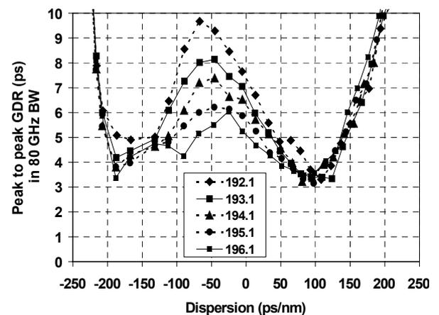
Figure 1. Measured peak to peak group delay ripple vs. dispersion setting for various channels (THz).
