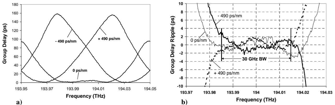
Figure 2. Group delay (a) and group delay ripple (GDR) (b) of 100GHz FSR device for different dispersion settings for the channel centered at 194THz. GDR is obtained by subtracting a linear fit of GD across the operating bandwidth.
