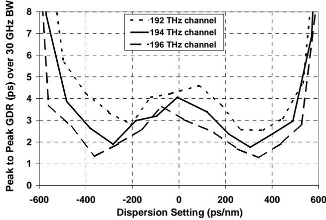
Figure 3. Group delay ripple (GDR) of 100GHz FSR device as a function of dispersion setting for 3 different channels. Note that GDR here is peak to peak and not +/-.
